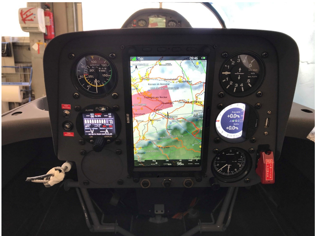
Suitable position for the FCU instrument Repeater on the rear panel of Duo Discus FES
