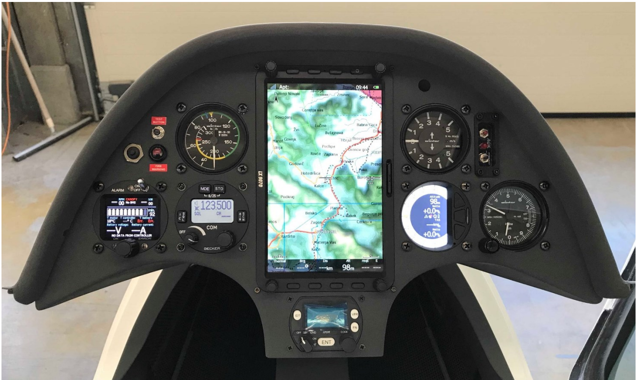
Suitable position for the FCU instrument Master on front panel of Duo Discus FES
